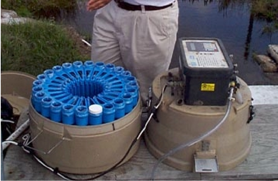
Figure 3.14. Automatic water sampler with plastic bottle liners.
