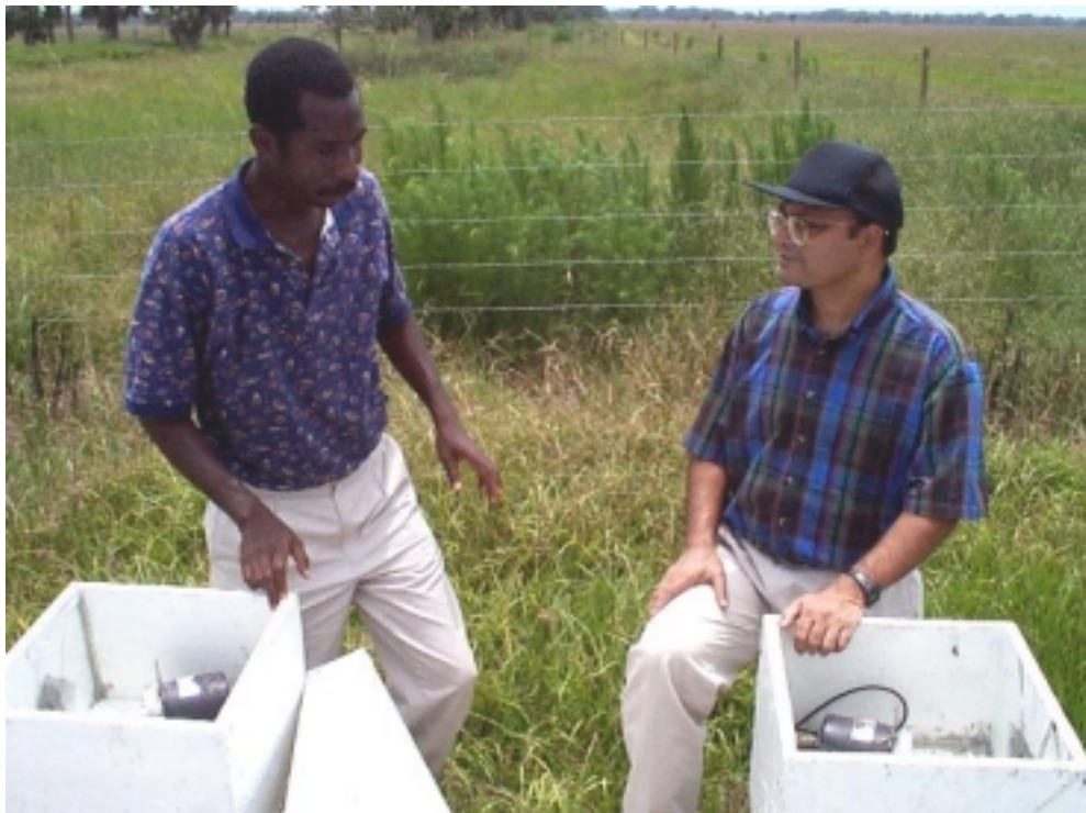
Figure 3.9. Digital stage encoders at stilling wells.
